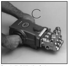
Separating Manifold Head from Crankcase
