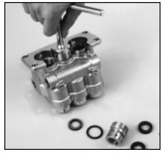
Removal of Seal Cases from Manifold Head
