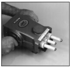
Proper Alignment of Ceramic Plungers for reassembly
