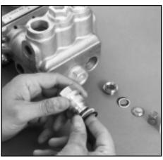
Examination of O-Ring and Back-up-Ring on Valve Plug
