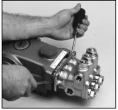
Removal of Manifold Head from Crankcase
